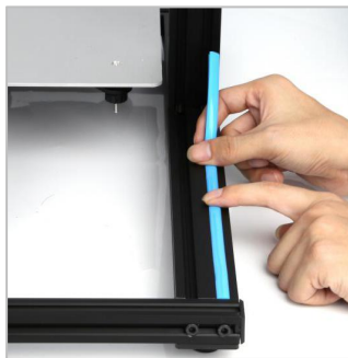
Install decoration belt into the notch, starting from one end.
